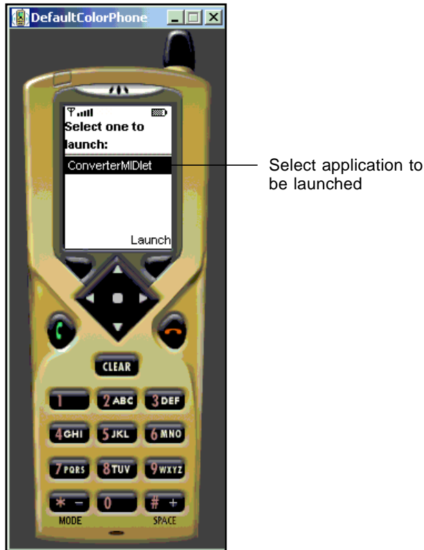
FIGURE 1-4 Testing a MIDlet Using an Emulator
